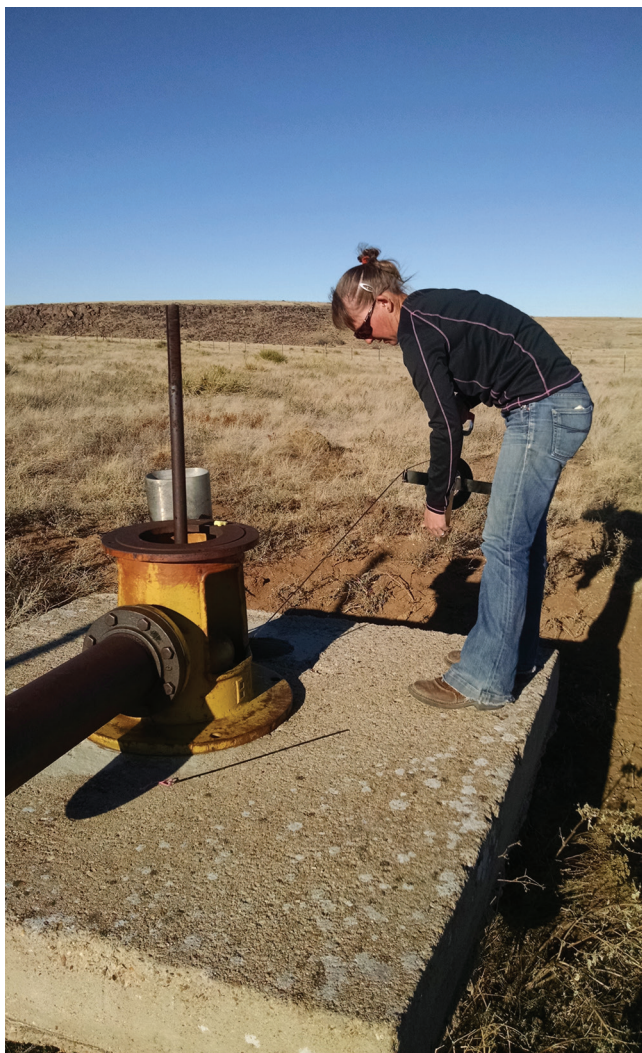
Figure 2. Using a steel tape in an irrigation well in Union County. (Photo courtesy of K. Ziegler.)
