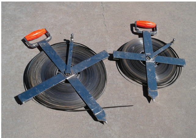
Figure 1. A 500-ft (left) and 300-ft (right) steel tape. (Photo courtesy of K. Ziegler.)
