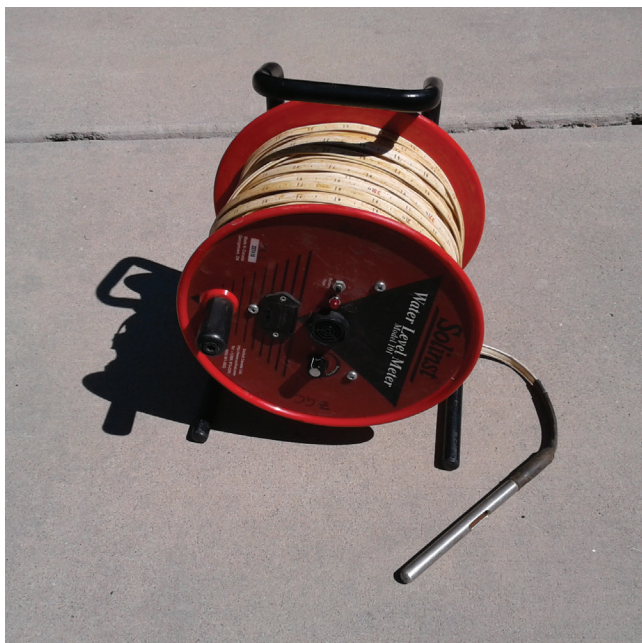
Figure 3. A 300-ft electric sounder or e-tape with its probe. The small hole in the middle of the probe contains the ends of the wire that run through the length of the tape. (Photo courtesy of K. Ziegler.)
