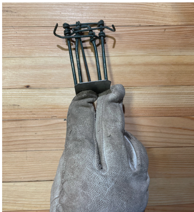
Figure 8a and 8b. Place fingers behind the pan to keep the trap from firing during placement.
