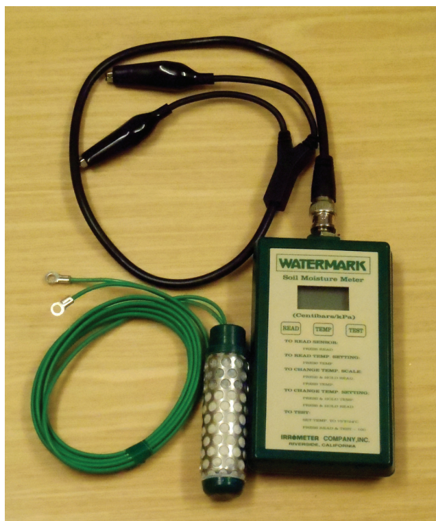
Figure 2. Granular matrix sensor and electric resistance meter.
