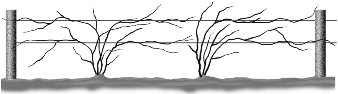
Figure 1. End posts for the trellis should be 4–6 inches in diameter and well anchored in the soil (2 feet deep). Stakes between the ends can be made of fence posts at least 18 inches deep in the ground. Treat all wood posts with a wood preservative. For organic growers, metal posts can be used for trellis.
