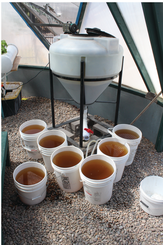
Figures 5a and 5b. Left: Aerobic mineralization tank used to provide dissolved nutrients from fish sludge to hydroponically grown plants. Right: Cucumbers grown entirely on nutrient solution derived from mineralization tank. Santa Fe Community College (SFCC), New Mexico, USA. (Photos courtesy of R. Shultz.)
