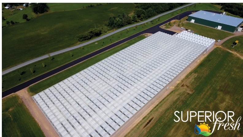
Figure 4. Aerial view of a large-scale commercial decoupled aquaponics operation showing the hydroponics section (left) separated from the fish house (right). Wisconsin, USA. (Photo courtesy of Superior Fresh.)
