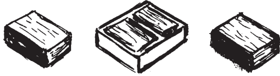
Figure 4. Loose adobe bricks (left and right) and adobe bricks in form (center).
