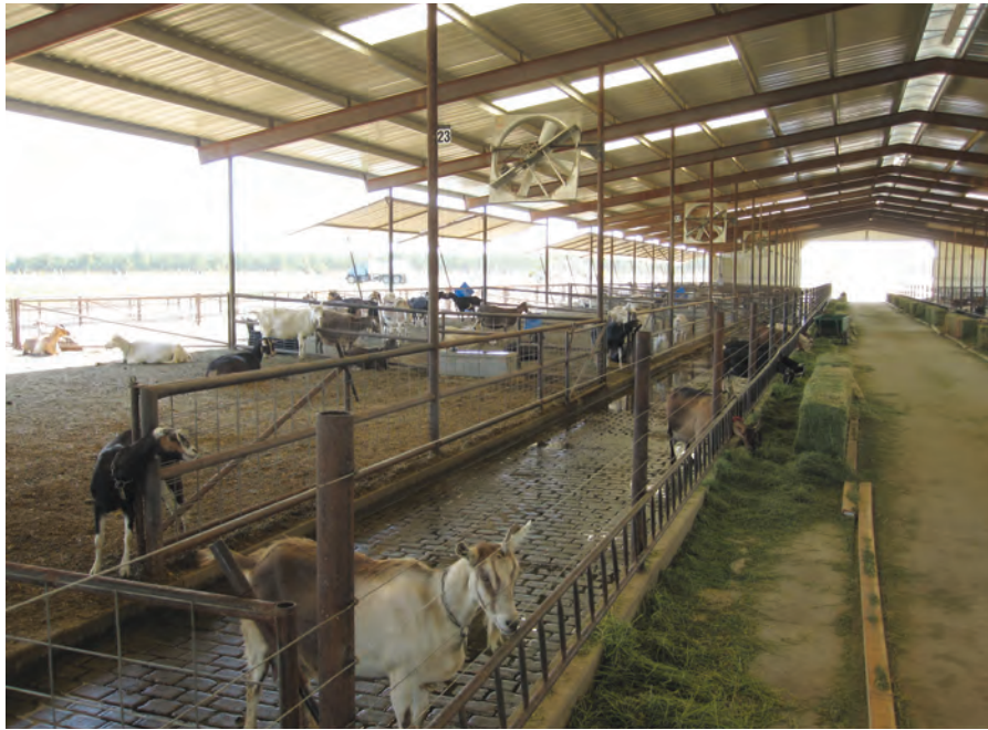
Figure 3. Automatic water troughs are provided in between pens. Fans are installed in this facility to provide additional airflow for goat comfort in the summertime. Also note the grooved concrete design in the feed alley to provide better traction for the animals.
