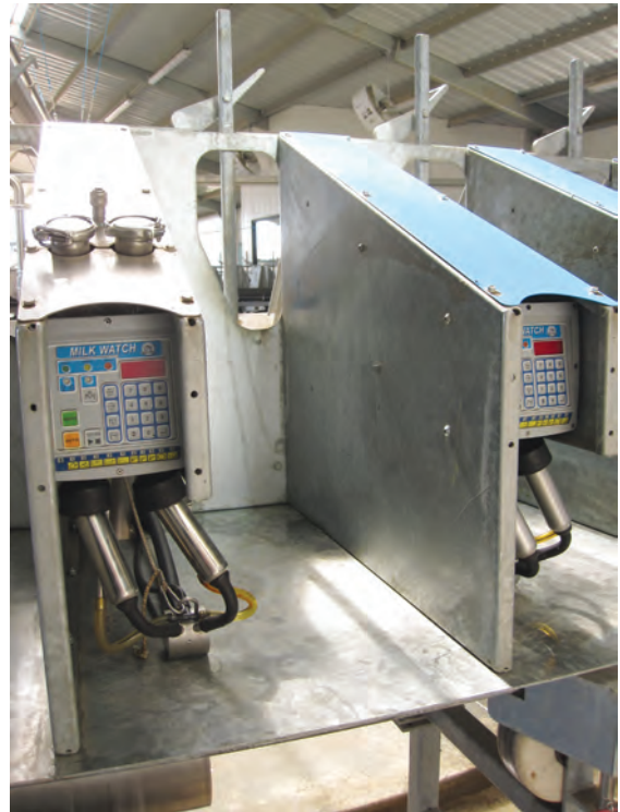
Figure 8. A modern milking station with computerized milk metering.
