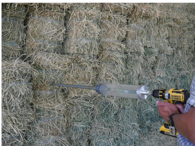
Figure 1. Proper sampling location on rectangular bales. Small 2-string bales shown here. Photo credit: Mark Marsalis.
