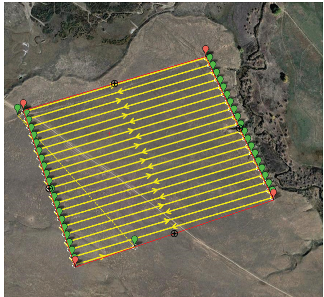
Figure 2. Drone flight path in a parallel survey grid with 75 percent side overlap.
