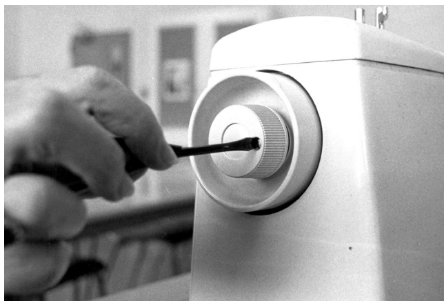
Figure 7. Handwheel area. Loosen screw in the face of the locknut in order to remove the clutch and handwheel.
