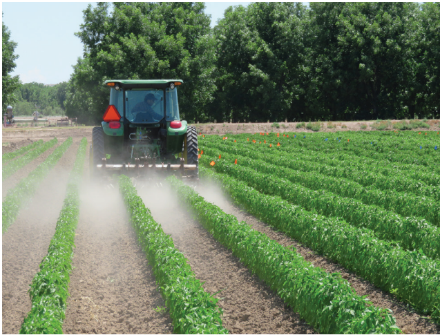
Figure 3. Using cultivation to control weeds in Chile, an example of mechanical pest control.
