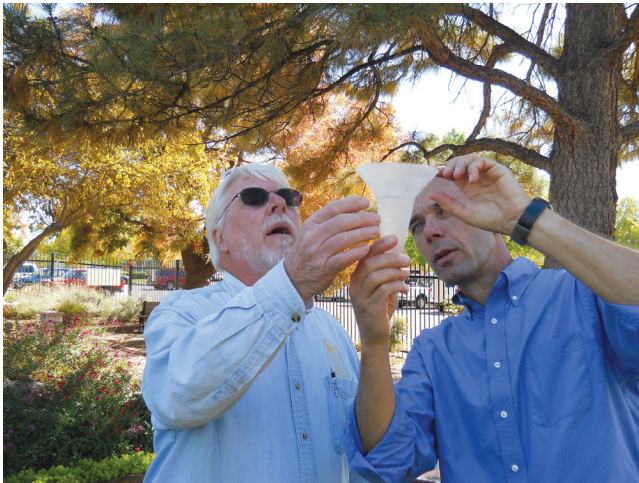
Figure 2. If graduated catch cans are used for irrigation audit, the graduated cylinder from Figure 1 is not needed and the volume may be read directly from the catch can.
