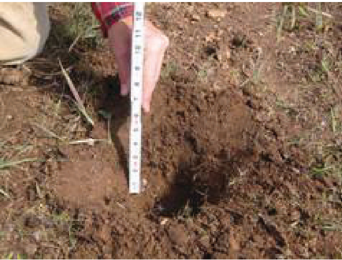
Figure 9. Measuring soil moisture in a 12-in.-deep soil pit.
